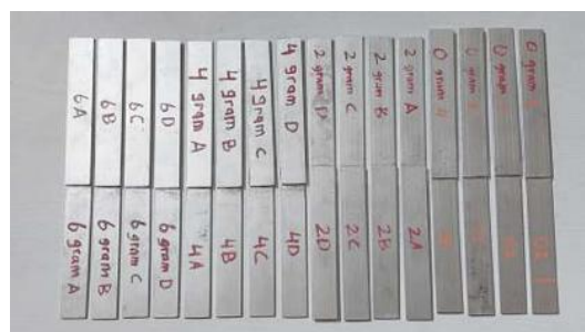
Figure 2. polyurethane adhesive-bonded aluminum single-lap joint specimens
