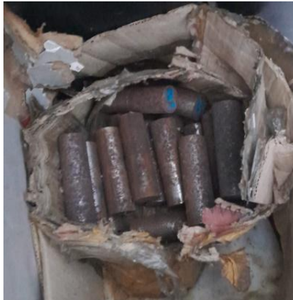
Gambar 2. Material Baja ST60
