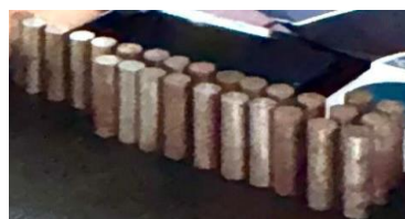
Gambar 1. Benda uji bermaterial ST 37
