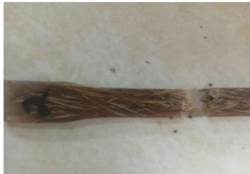
Gambar 6. Patahan sampel uji tarik 35%
