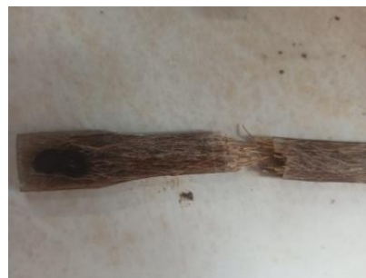
Gambar 8. Patahan Sampel Uji Tarik 45%
