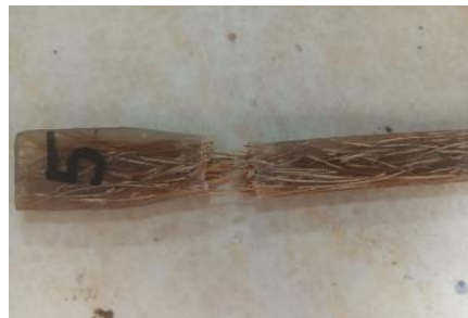
Gambar 7. Patahan Sampel Uji Tarik 40%
