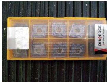
Gambar 2. Insert Carbide Mitsubishi CNMG 120408-MA
