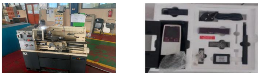
(a) Mesin Bubut Bemato Seri 44378 (b) Surface Roughness Tester type Mitutoyo SJ-210 Gambar 2. Peralatan Penelitian
